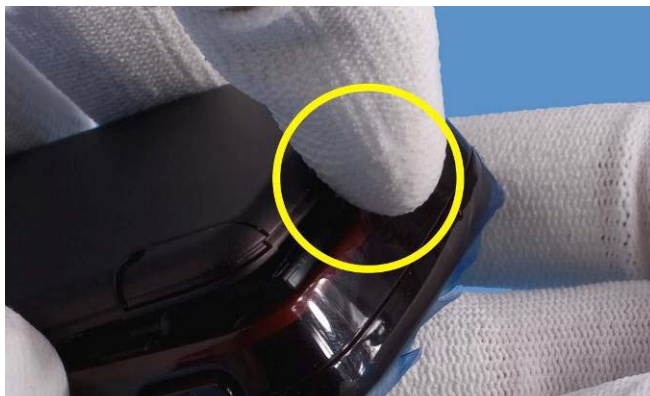
1. Press to release the BATTERY COVER .
