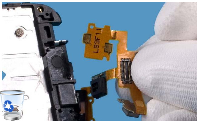
33. Remove UPPER FLEX ASSY . UPPER FLEX ASSY has always to be renewed.
