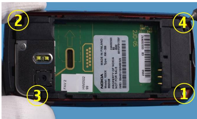
3. Unscrew the four TORX5+ screws.
