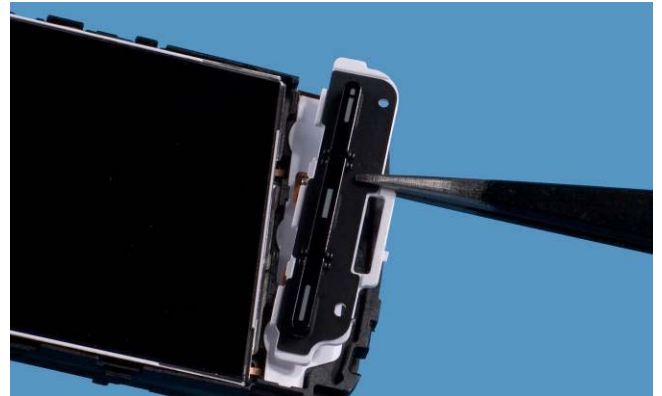
14. Use tweezers to remove KEYMAT .
