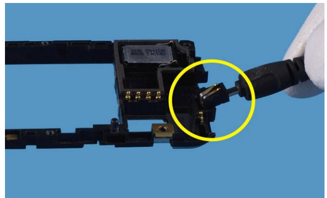
34. Remove CONN CHR DIA 2.0mm with a DC-plug.
